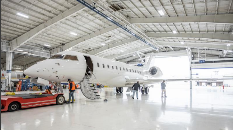
The first of three Bombardier Global 6000 is undergoing comprehensive structural modifications to accommodate the HENSOLDT Kalatron SIGINT payload
